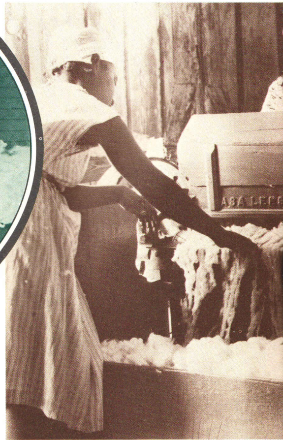
The mechanical gin these women are using to separate the seeds from the fibres has changed very little since the 18th Century.
